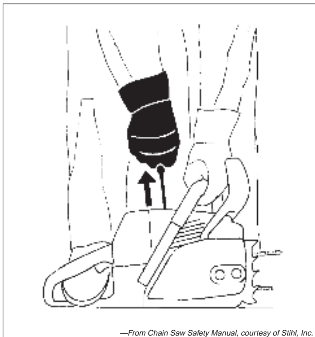
Figure 2-17—Start the saw on firm ground.
