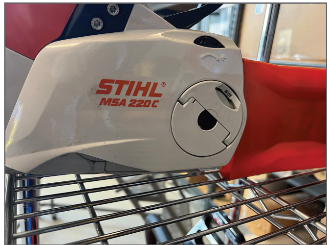
Figure 9—A chain quick-tension dial found on three of the seven saws tested.
