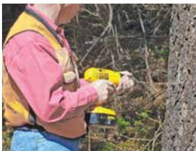
Fig. 8 – Battery-powered drills can be used to check for sound-rind thickness.
