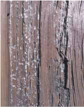
Fig. 38 – Wood with decay caused by Phellinus pini , commonly called whitespeck, is relatively sound compared to wood decay caused by other fungi.
